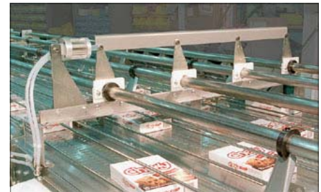
Pneumatically Actuated QuickSet® Guides on AIR DECK®
