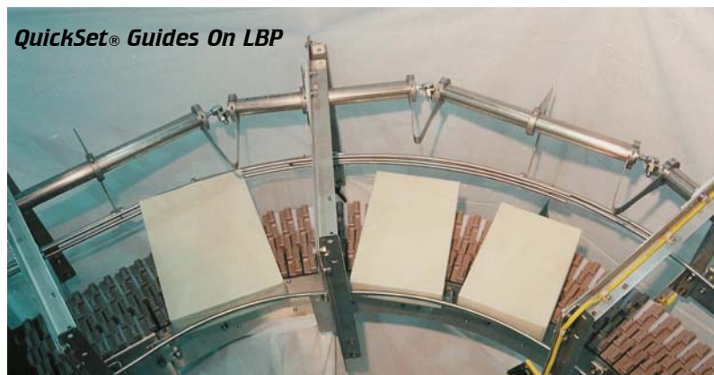
Pneumatically Actuated QuickSet® Guides on AIR DECK®
